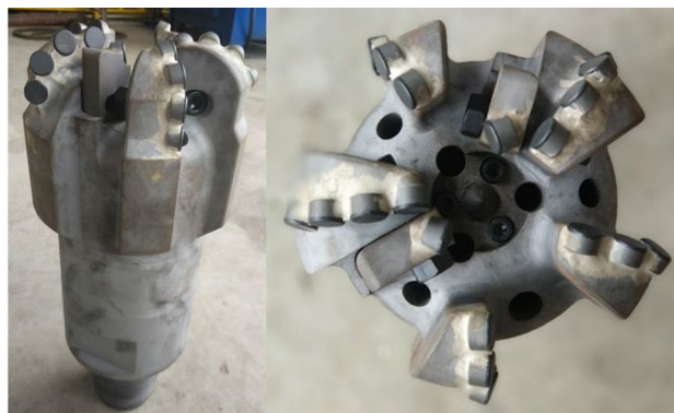
Fig. 15 The micro-coring PDC test bit
