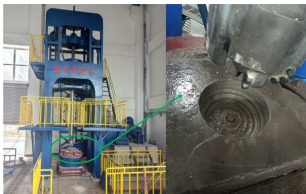
Fig. 16 Drilling process of the test bit
