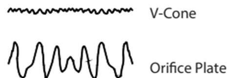
Fig. 11 DP Meter signal stability (McCrometer 2013)
