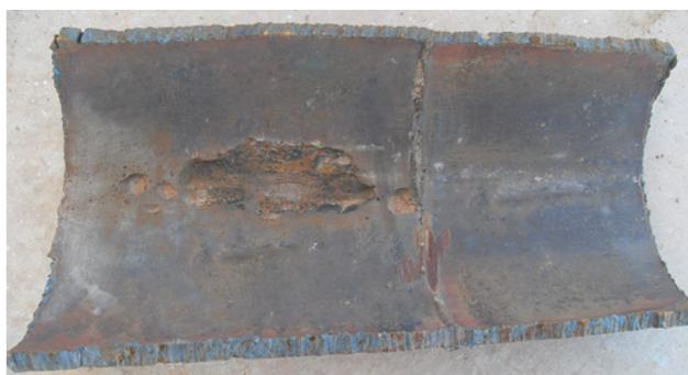
Fig. 2 Internal piercing of carbon steel flow line
