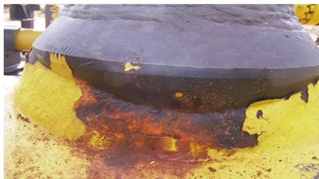
Fig. 3 Visual inspection of corroded pipe
