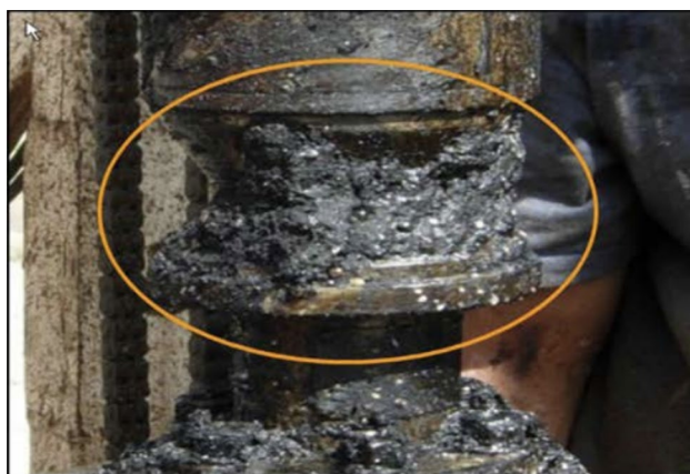
Fig. 8 Asphaltene Solid Deposit on the Surface of ESP (Jennings et al. 2020)
