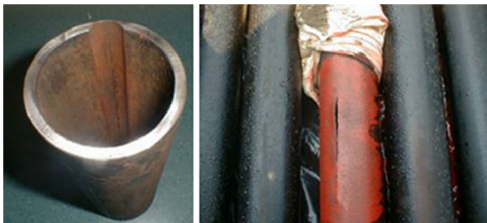
Fig. 12 Tubing failure example (Langbauer et al. 2021)
