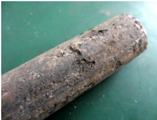
Fig. 18 Corrosion failure in the beam rod pump downhole components (Zhang et al. 2020)
