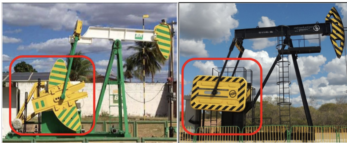
Fig. 7 Conventional and smart sucker rod pump (Oliva et al. 2020)
