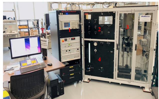
Fig. 3 AutoLab 1500 for permeability and ultrasonic measurements: (1) Digital panel (2) Controlling valves (3) Core holder and core assembly (4) Pressure intensifiers
