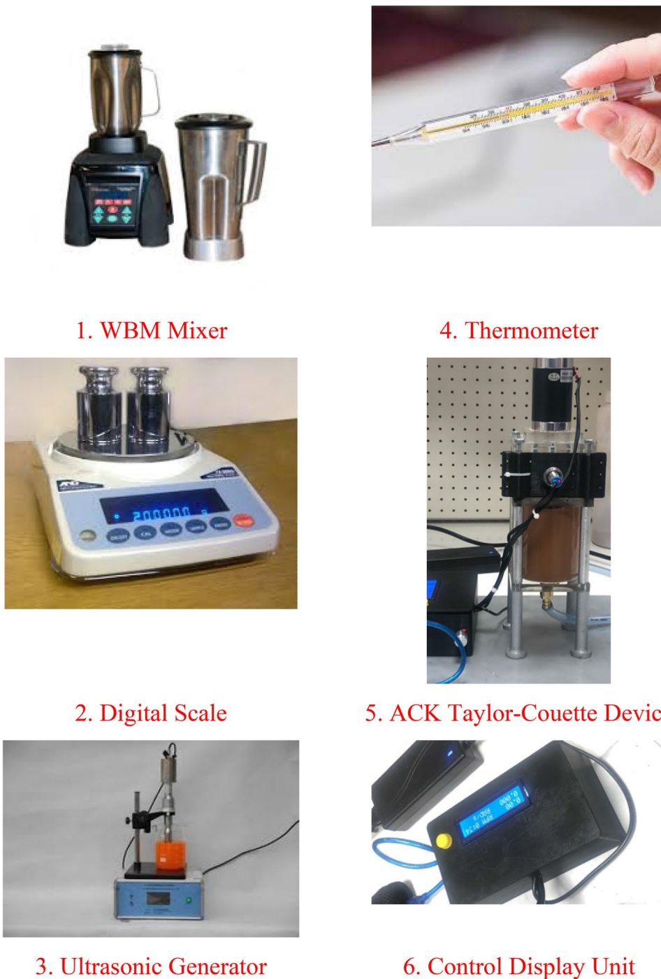
Fig. 4 Steps for preparing and testing WBM nanofluids in the ACK TCS (Rashidi et al. 2020a)
