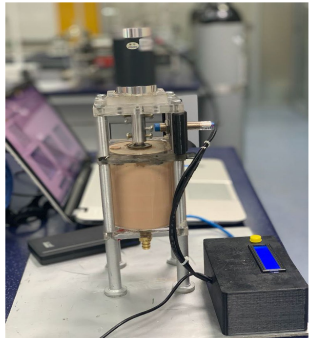
Fig. 1 ACK Taylor–Couette system (TCS) (Rashidi et al. 2020a)
