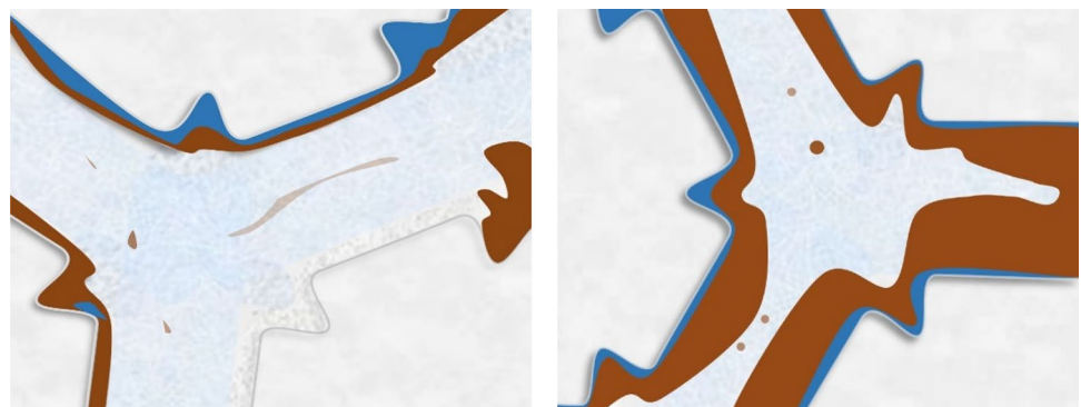
Fig. 6 Microscopic analysis of surfactant flooding in left water-wet medium and right oil-wet medium. The deep blue is representative of the formation brine, the brown represents the oil, and the white represents the surfactant solution (Yadali Jamaloei and Kharrat 2009 adapted from Yadali Jamaloei and Kharrat (2009))
