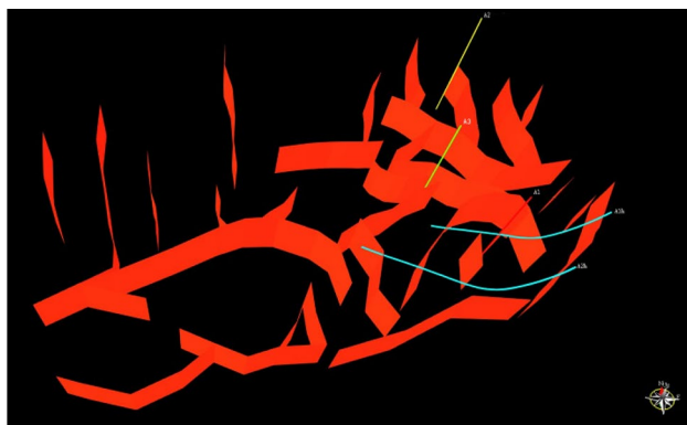
Fig. 11 Spatial distribution of large-scale cracks based on the TFL attribute recognition
