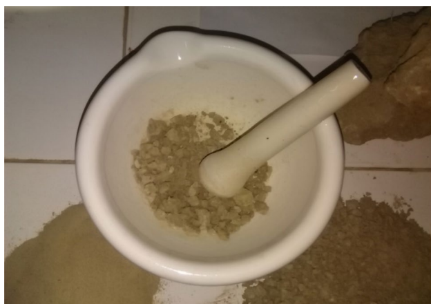
Fig. 4 Mortar and pestle been used to crush clay material
