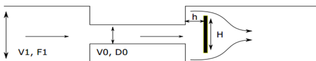
Fig. 4 Initial design of flow around a disk pig to calculate the pressure drop at the two sides of the pig (Ref. (Idelchik 1987))
