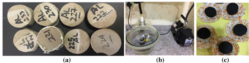
Fig. 1 a Core plugs after drying. b Saturating core plugs with crude oil. c Cores after saturation
