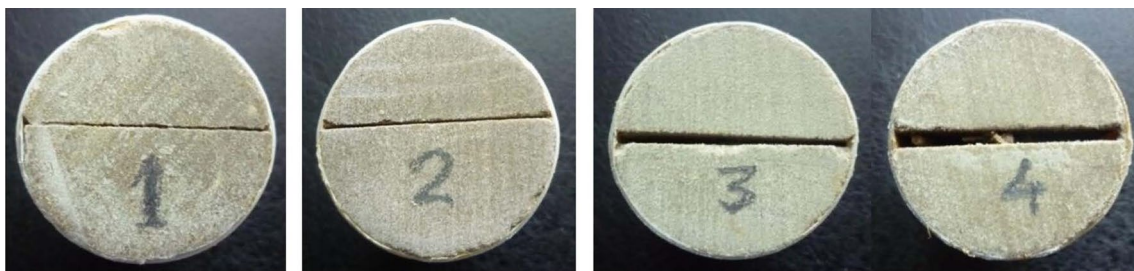
Fig. 2 Top face of the fractured core plugs
