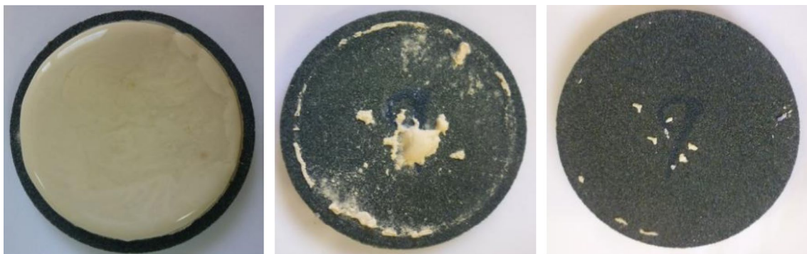
Fig. 6 Demonstration of wellbore cleaning efficiency by the clean-up fluid composition. Initial cake (left); remaining cake after enzyme treatment (center); remaining cake after acetic acid treatment (right)
