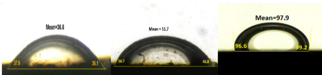
Fig. 16 Contact angle of water drop on rock pellet that was aged in surfactant solution by combination with 6 \text{So}_4^{2-} (left), 6 \text{Ca}^{2+} (middle) and 6 \text{Mg}^{2+} (right)
