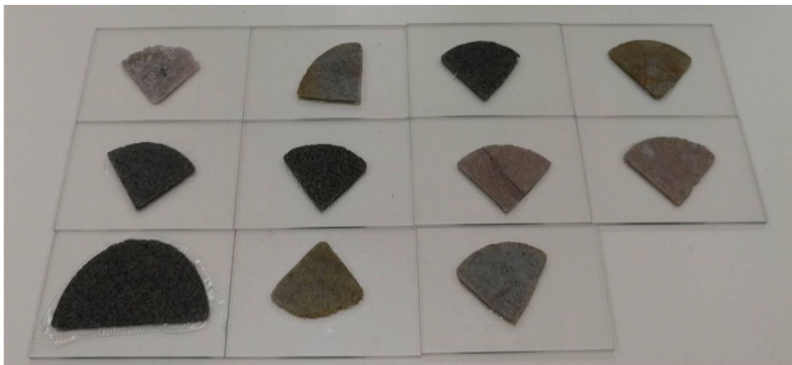
Fig. 2 Core samples prepared for wettability analysis
