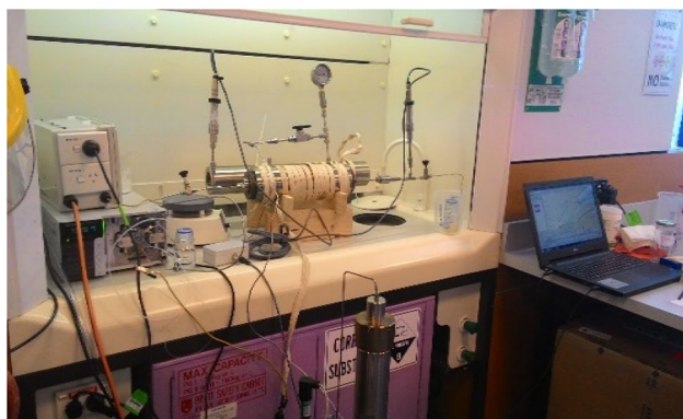
Fig. 3 Core flood setup
