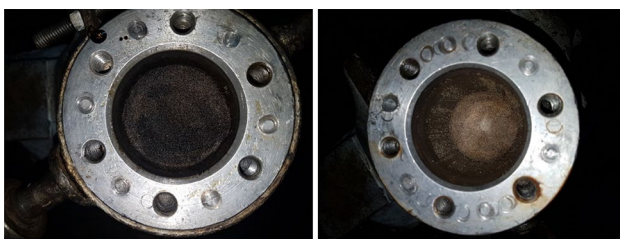
Fig. 11 Photographs of sandpaks after flooding with sea water (left) and the emulsion 60/40 (right)
