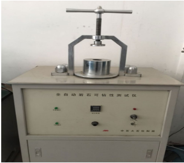
Fig. 1 Fully automatic rock drilling test instrument
