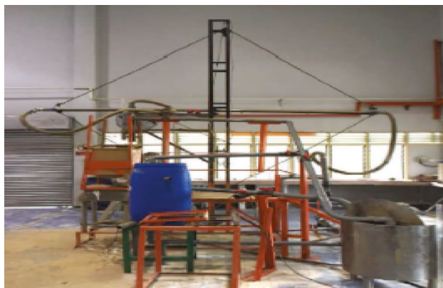
Fig. 4 Layout of the cuttings transport flow-loop
