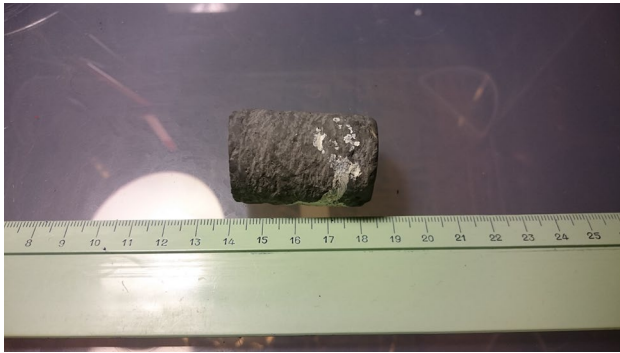
Fig. 4 Rock sample used for pyrolysis analysis
