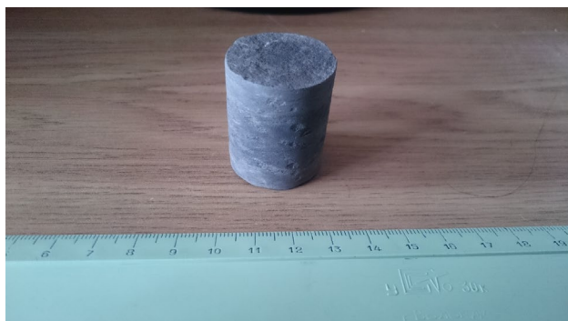
b core sample from the Paleocene deposits of Well # 7 Blagodarnenskaya, used to measure resistivity at 100% water saturation
