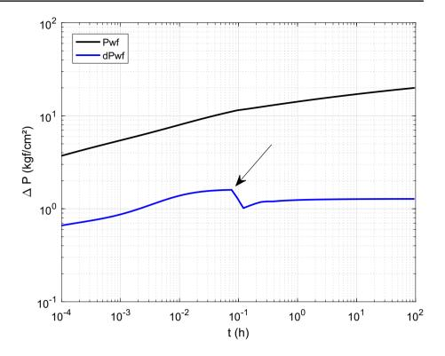
**Fig. 2** Pressure and derivative data for case B
