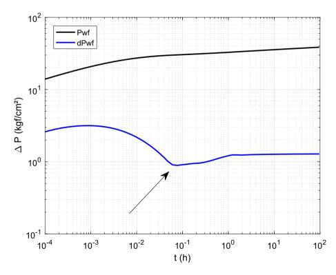
Lastly, skin zone permeability might be determined through Eq. (1), applying the previously computed values for the mechanical damage and skin radius. Reservoir permeability, which is also required by Eq. (1), is estimated from the constant pressure derivative level (Banerjee et al. 1998; Bela et al. 2019):
