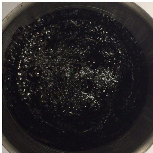
Fig. 13 CO 2 dissolved in the crude oil being liberated
