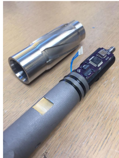
Fig. 3 Downhole sensors in the BHA
