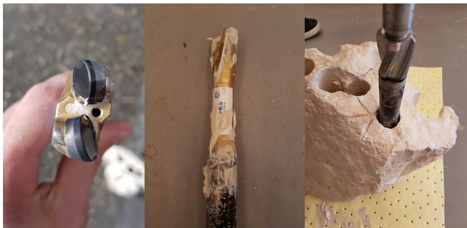
Fig. 8 From left: Plugged nozzle, bit balling paste, well hole diameter being on gauge with bit diameter
