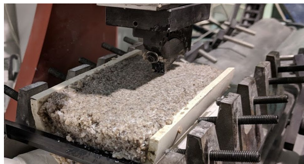
Fig. 6 Scratch test performed on 2-mm sand
