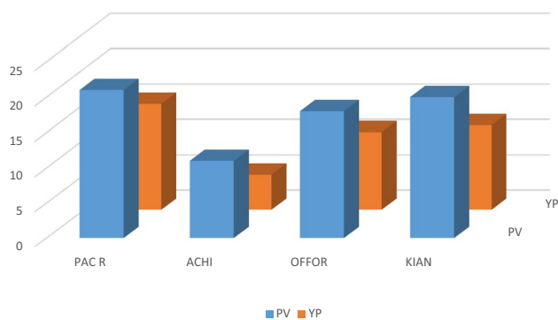
Fig. 3 Flow properties of the water based mud for each viscosifier at 120 °F
