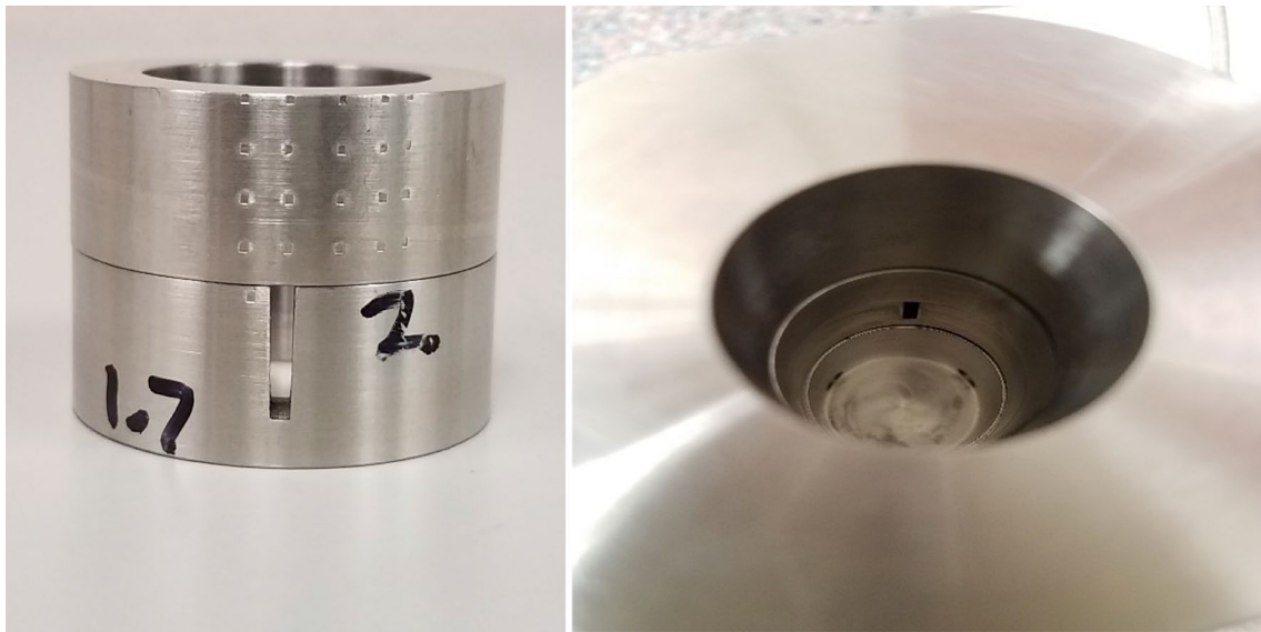
Fig. 6 2000- \mu\text{m} -width fracture slot (left) and well-secured fracture slot in a core holder (right)
