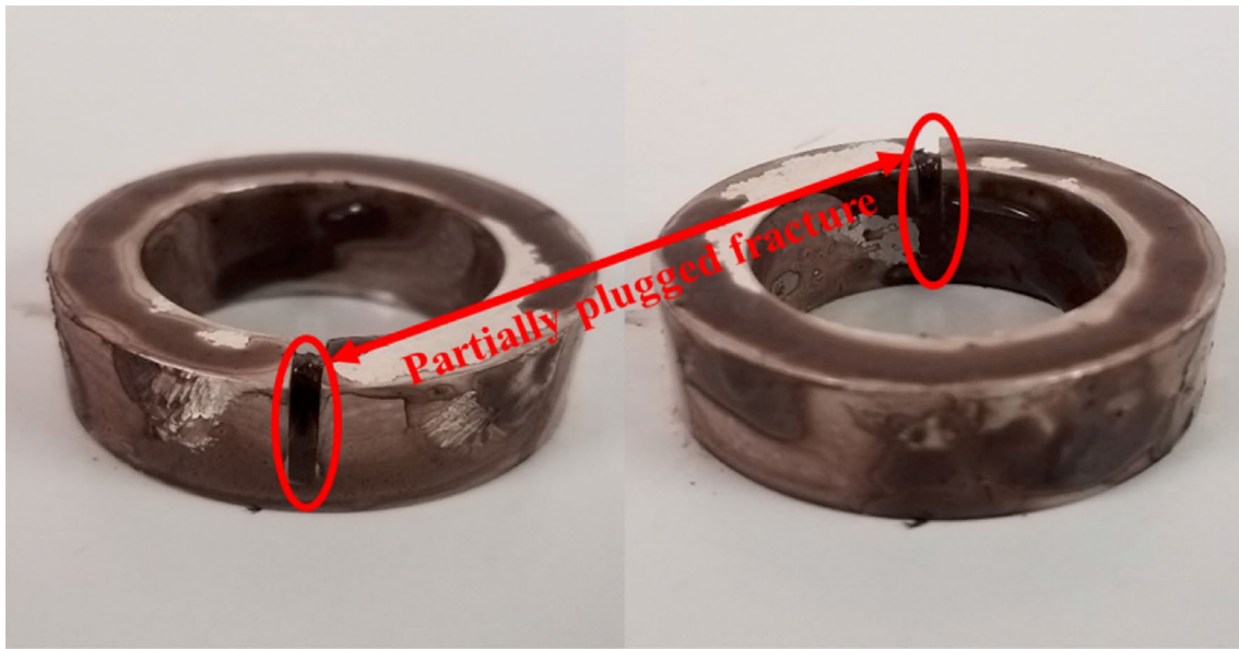
Fig. 18 Plugged fracture core slot after the polymer/fiber blend dynamic fluid loss test at 120 °F
