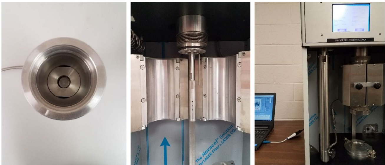
Fig. 7 Core holder with slot placed inside a mud cylindrical holder (left). Rotating shaft, temperature sensor and heating bath (middle). Complete setup of the dynamic mud loss experiment (right)
