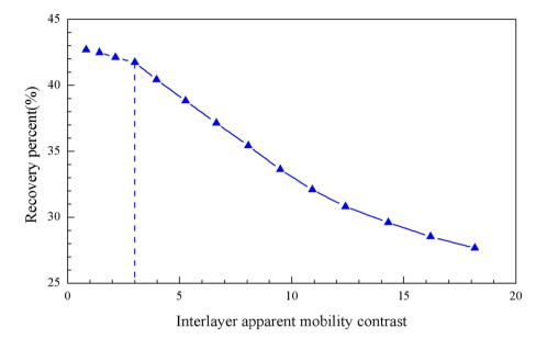
pressure drop, keeping apparent mobility contrast within 3.0 is the policy limit for layer recombination of this low-permeability reservoir at 90% water cut.
