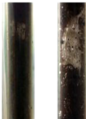
Fig. 3 Comparison between the mixing of heavy oil and light oil with gas injection and without gas injection
