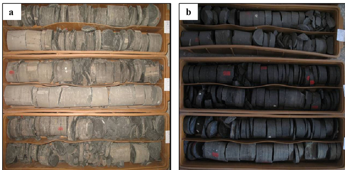
Fig. 9 Mudstone of the X–XII sand groups of the K_2qn^3 Formation in the Daqingzijing oilfield. a Gray-black mudstone in the Qian157-19-9 well core data, b black mudstone in the Hei120 well core data
