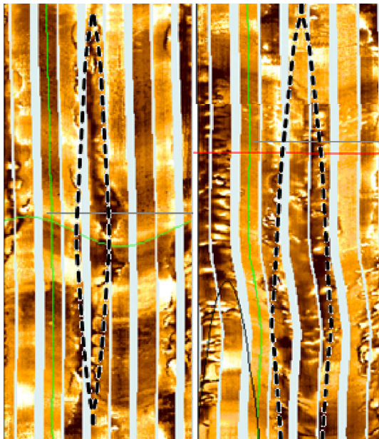
Fig. 6 Compression of calculated ( dash line ) and observed breakout widths in different depths of the wellbore
