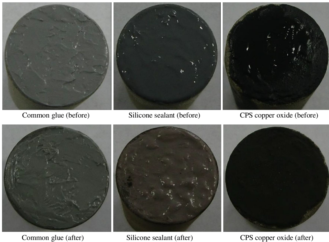
Fig. 10 Comparison of three kinds of glues before and after heating
