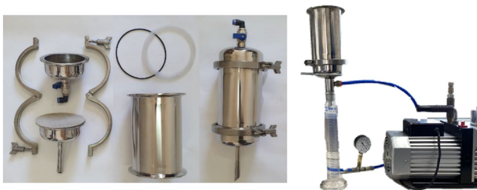
Fig. 1 The vacuum pump and the main components of Büchner funnel used in vacuum filtration system
