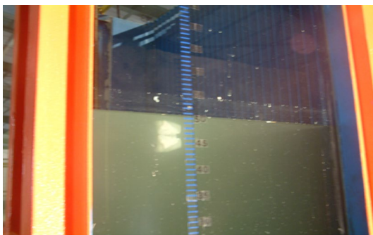
Fig. 7 Graduated wall of the reservoir in order to measure of the water level
