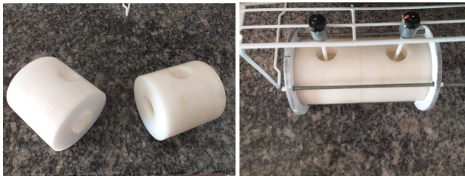
Fig. 2 Membrane reactor used in transport of Methylene Blue (MB)
