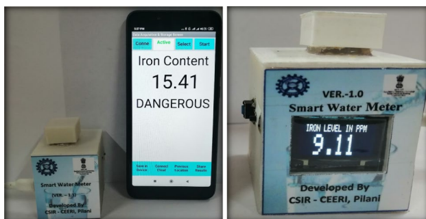
Fig. 6 Developed handheld IoT-enabled and standalone spectrometer system for offline heavy metal measurement
