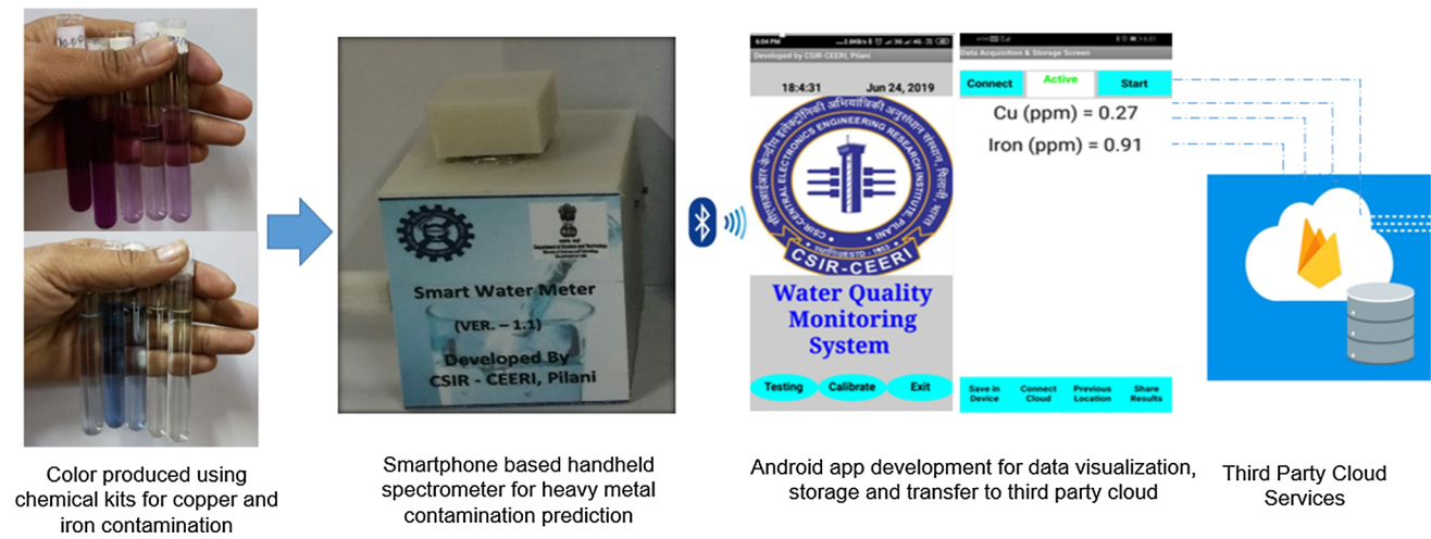
Fig. 7 Overall flow of developed IoT-enabled handheld spectrometer system for heavy metal (Fe and Cu) contamination prediction
