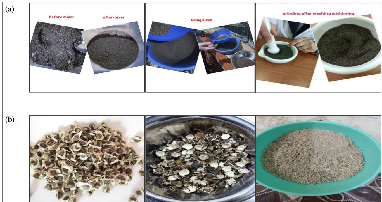
Fig. 1 preparation of a olive pomace adsorbent material b Moringa seeds Husks adsorbent material
