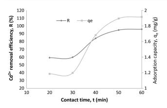
**Fig.6** Effect of contact time on the adsorption of  $Cd^{2+}$  onto Cu-MOF at adsorbent dose=0.5 g/50 mL, initial  $Cd^{2+}$  concentration=20 mg/L, pH=4.0 and temperature=30 °C
