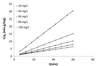
Fig. 10 Pseudo-second-order model for adsorption of Cd<sup>2+</sup> onto Cu-MOF at different initial concentrations
