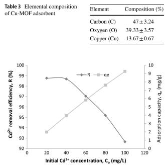
**Fig. 5** Effect of the initial  $Cd^{2+}$  concentration on the adsorption of  $Cd^{2+}$  onto Cu-MOF at adsorbent dose=0.5 g/50 mL, contact time=60 min, pH=4.0 and temperature=30 °C
