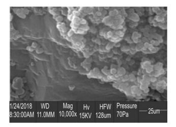
Fig. 3 SEM image of as-synthesized Cu-MOF adsorbent
