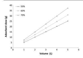
Fig. 12 Adsorbent dose (W) against treated Cd<sup>2+</sup> solution volume (V) at different removal efficiencies
