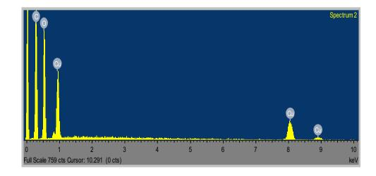
Fig. 4 EDX spectrum of Cu-MOF adsorbent
