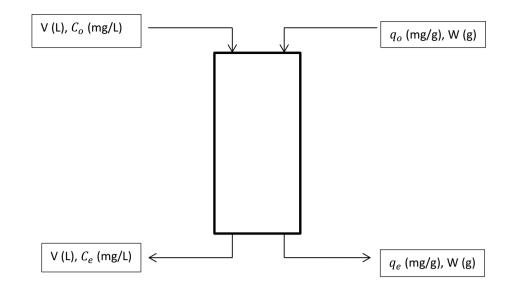
is fed into the adsorber containing the effluent and the amount of  $Cd^{2+}$  adsorbed at equilibrium changes from  $q_0$  (it is zero initially) to  $q_e$ .
