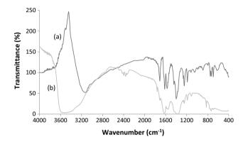
Fig. 2 FTIR spectra of the prepared MOF a without  $Cd^{2+}$  adsorption and b with  $Cd^{2+}$  adsorption
