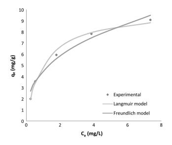
Fig.8 Two-parameter isotherm models for adsorption of  $\rm Cd^{2+}$  onto Cu-MOF adsorbent at 30  $^{\circ}\rm C$
