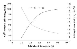
**Fig. 7** Effect of adsorbent dosage on the adsorption of  $Cd^{2+}$  onto Cu-MOF at initial  $Cd^{2+}$  concentration=20 mg/L, contact time=60 min, pH=4.0 and temperature=30 °C
