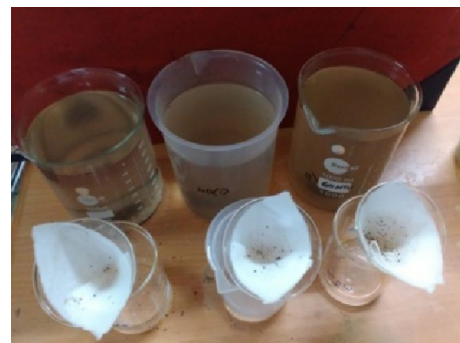
Fig. 4 Flocculation–coagulation with seeds powder filtration
