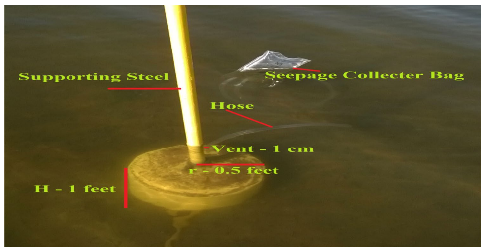
Fig. 2 Manual seepage meter established for the present study (modified after Lee 1977)
