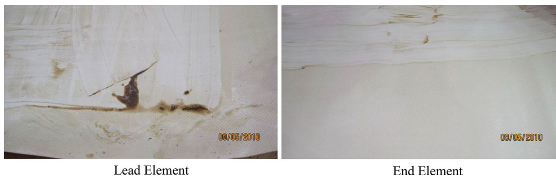
Fig. 6 Photographs of membrane elements used in baseline study—first trial—showing foulant deposits and scraped area
