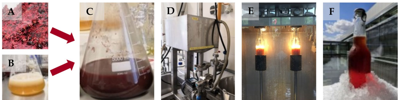
Fig. 1 Processing of the beverage: black currant pomace (A), pre-culture of W. cocos in malt extract medium (B), fermentation in shaking flasks (C), cross-flow filtration (D), filling into bottles (E), and produced beverage (F)
