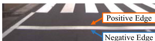
Fig. 8 Conceptual schematic of positive and negative edges
