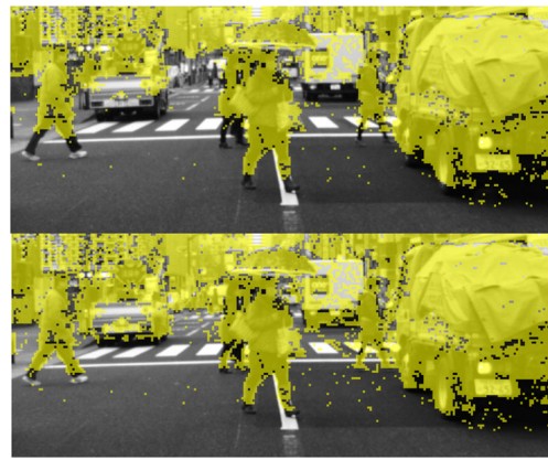
Fig. 8 The segmented obstacle surface locating above the ground level which is estimated by conventional method (top) and proposed method (bottom) at the 8th frame of the evaluation scene
