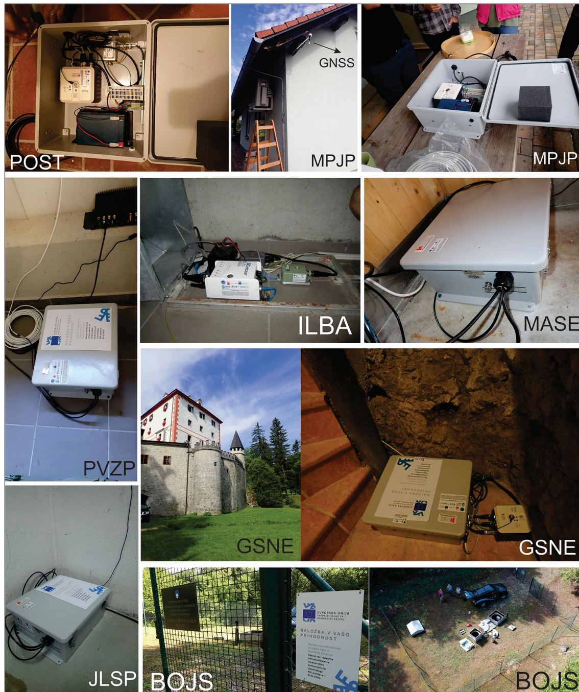
Fig. 3 Seismic research infrastructure for the SLO KARST NFO site (POST, MPJP, PVZP, ILBA, MASE, GSNE AND JLSP) and for Bojanci (SE Slovenia, BOJS) installed in 2020. Figure 1 gives locations of individual seismic stations. Photos S. Šebela, M. Krebelj, M. Mali and I. Tasič
