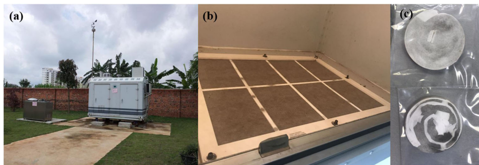
Fig. 1 a The aerosol collector is installed in the integrated automatic monitoring station, and the sampling port is approximately 2 m from ground level; b the inside of the aerosol collector where the filter membrane is placed; c the filter membrane, where the black areas are aerosols
