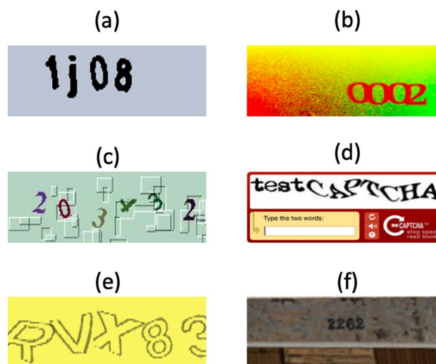
Fig. 1 Demonstrating some of the commonly used security features in securing text-CAPTCHA schemes: (a) Character isolated, (b) Overlapping, (c) Rotation and Random Noise, (d) Warping, (e) Hollow scheme, (f) Background as a noise
