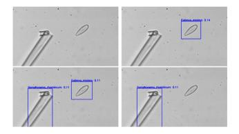
Fig.6 Detection flickering. Instances are detected and missing in consecutive frames with imperceptible differences in background noise
