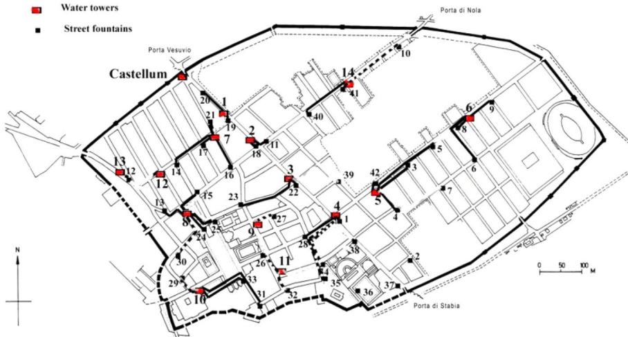
Fig. 1 Probable pipe connections to street fountains marked by solid lines and plausible connections by dotted lines. Drawing by author modified from Ray Laurence's base map in Laurence 1994
