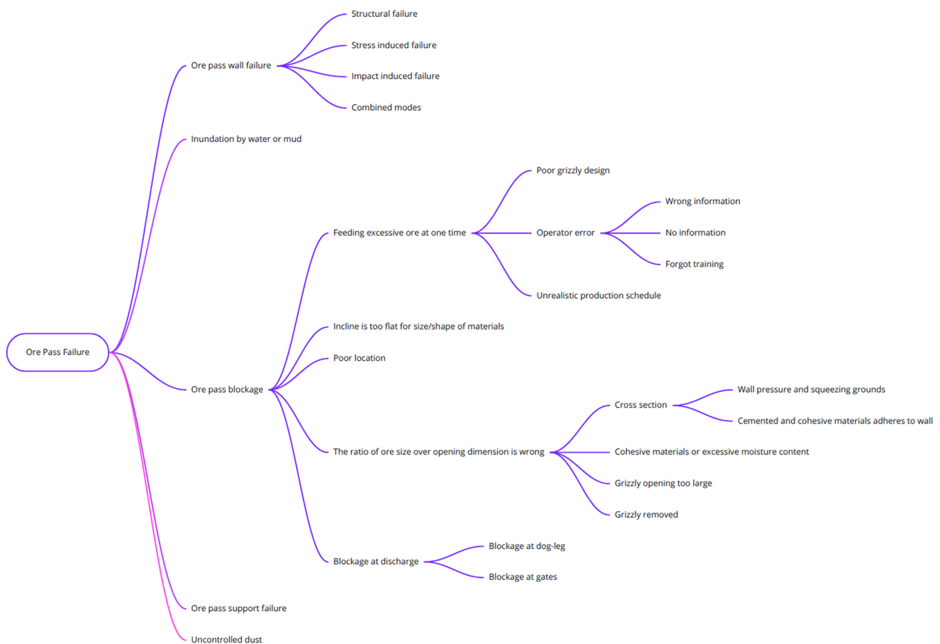
Fig. 12 A partial fault-tree diagram showing the main mechanisms of failure in ore passes (Adopted and modified from Beus et al. 1997)
