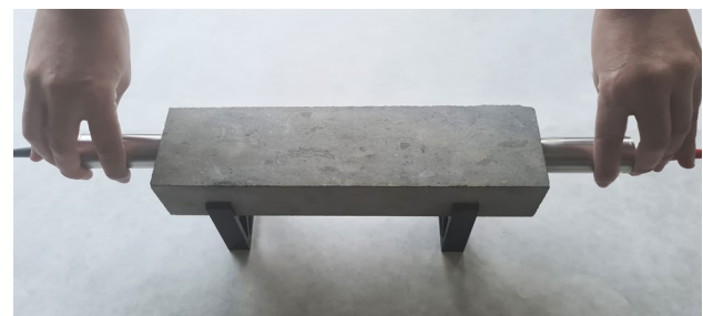
Fig. 6 Ultrasound propagation velocity test (X-axis direction)
