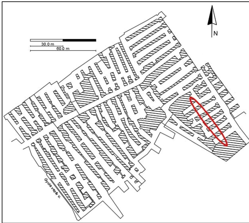
Fig. 4 Studied cellular system—the red colour refers to the studied cross section, the hatched area represents the pillars
