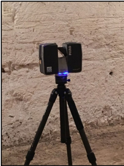
Fig. 7 Used TLS device, while it is working inside the cellar system
